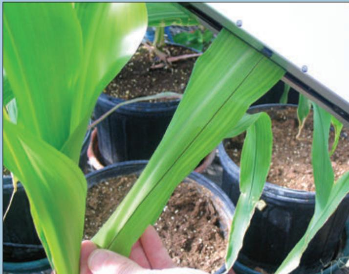
2) The closed scanning head is drawn over the leaf, allowing the leaf apex to pass through completely.
