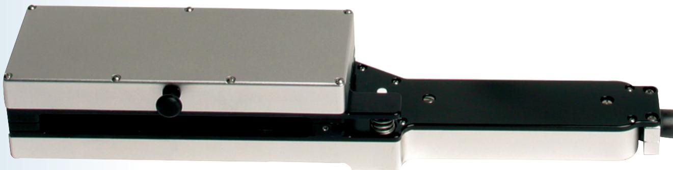
The LI-3000C provides a non-destructive, precise method to measure leaf area. Leaf area development or reduction associated with conditions of insect infestation, drought, disease or air pollution can be measured in the field or in growth chambers.
