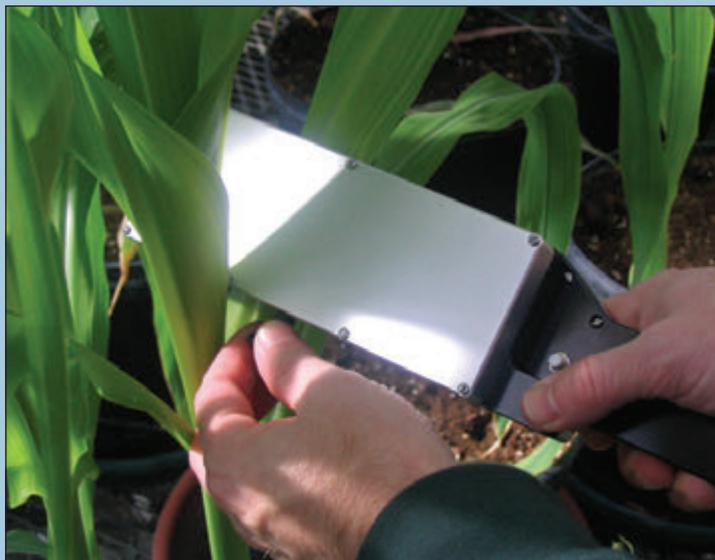
1) The scanning head is opened and placed over the leaf. The length encoding cord is held stationary against a stable object, usually the stem at the base of the leaf. The scanning head is closed at the base of the leaf and the reset button is pressed to initiate a new measurement.
